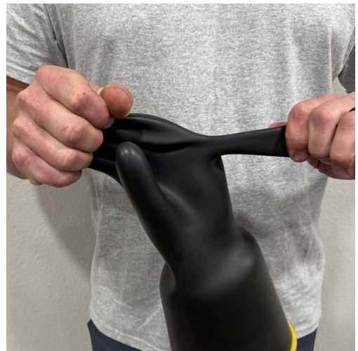
Figure 6-4 – Checking between the fingers, close up
